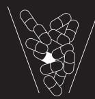
Feeding: The feeding system organizes the products into lines for stable and continuous inspection.
