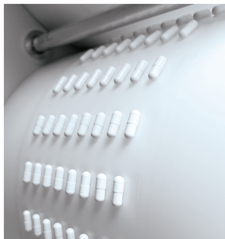
SPINE FIBO implements controlled manipulation of each product that allows 100% visual inspection and accurate counting before bottle filling
